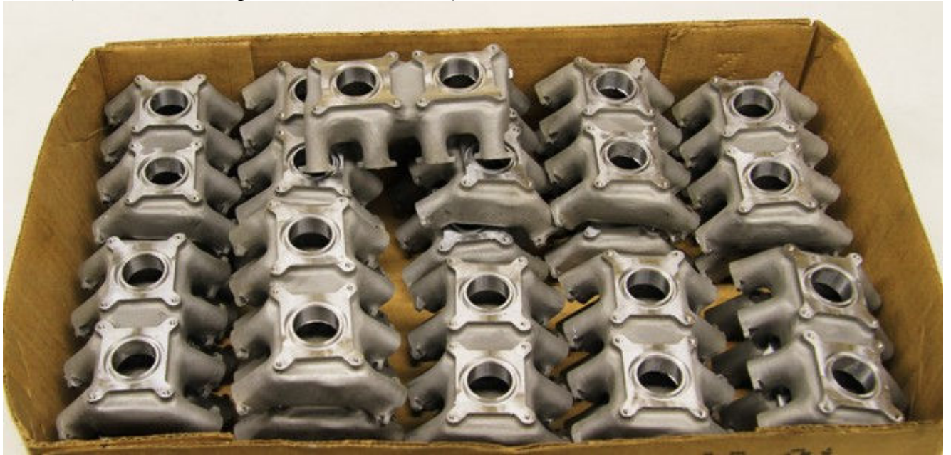
Pic #7 (22 additional completed intake manifolds)
