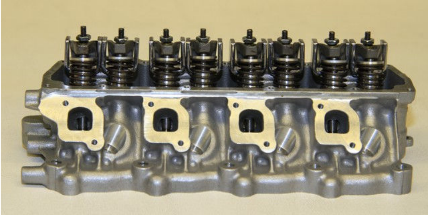
Pic #6 (Notice how rocker arms align with top of each valve)
