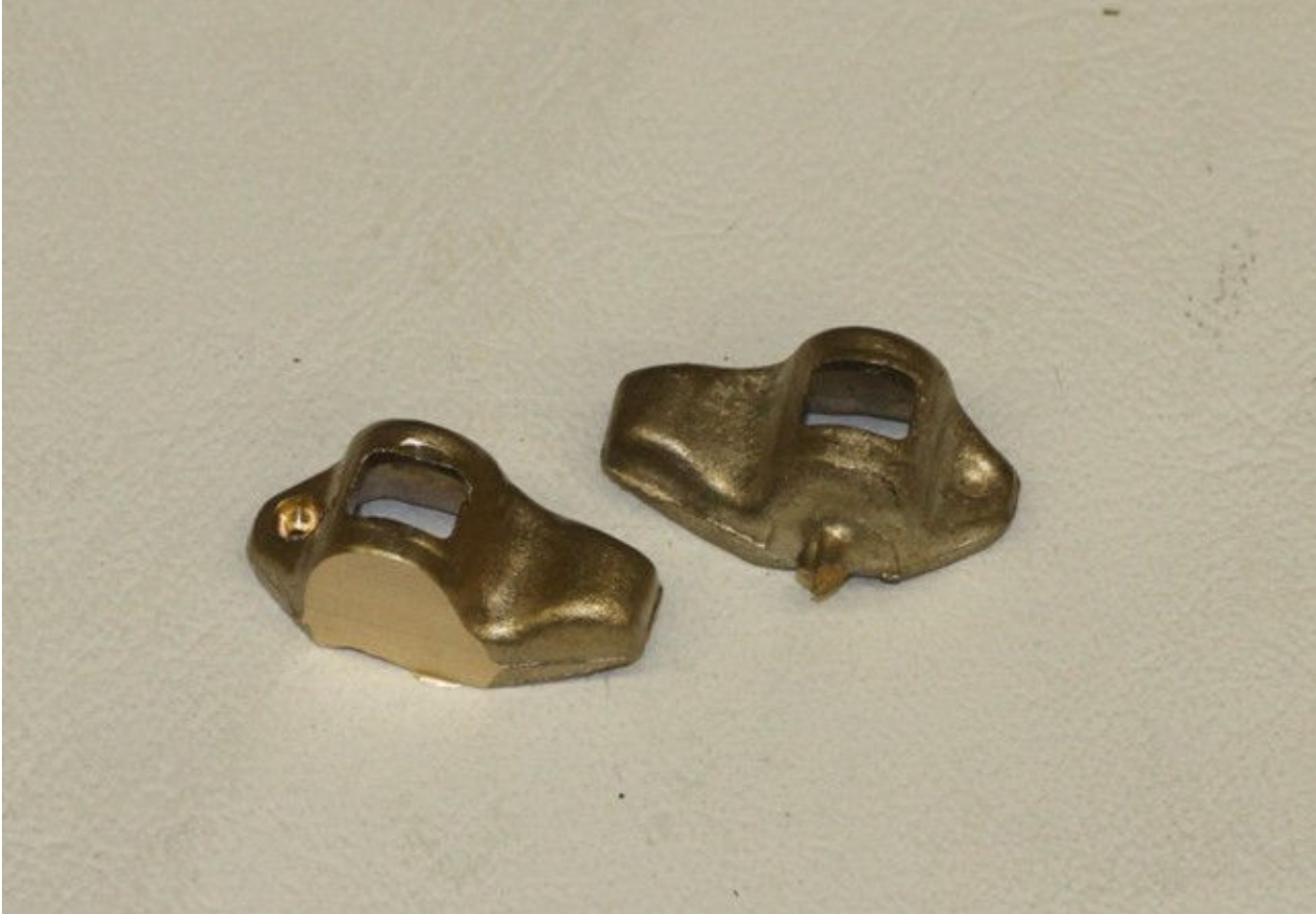
Pic #1 (Rocker arms – before on right, after on left)
