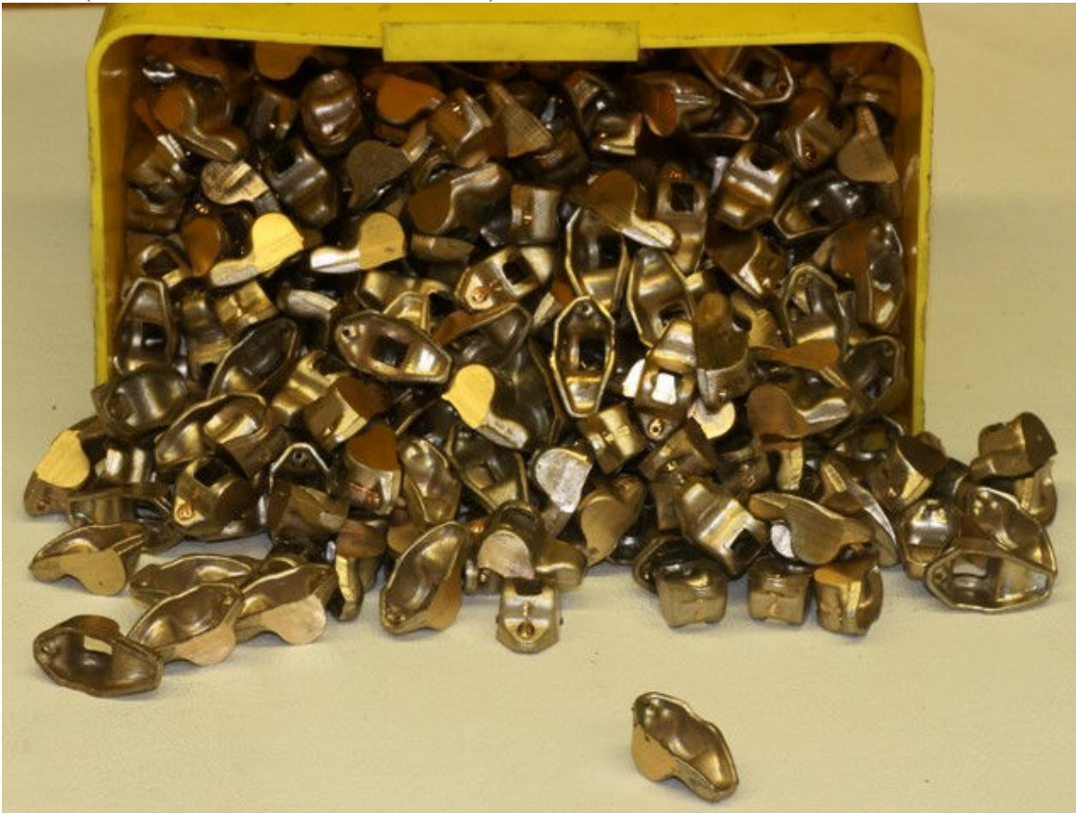
Pic #3 (Partial box of finished rocker arms)
