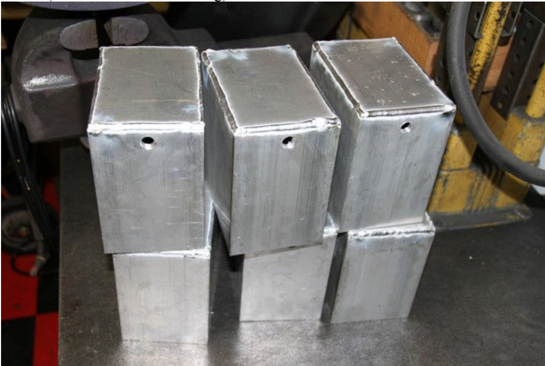
Pic #4 (Water tanks after welding)
