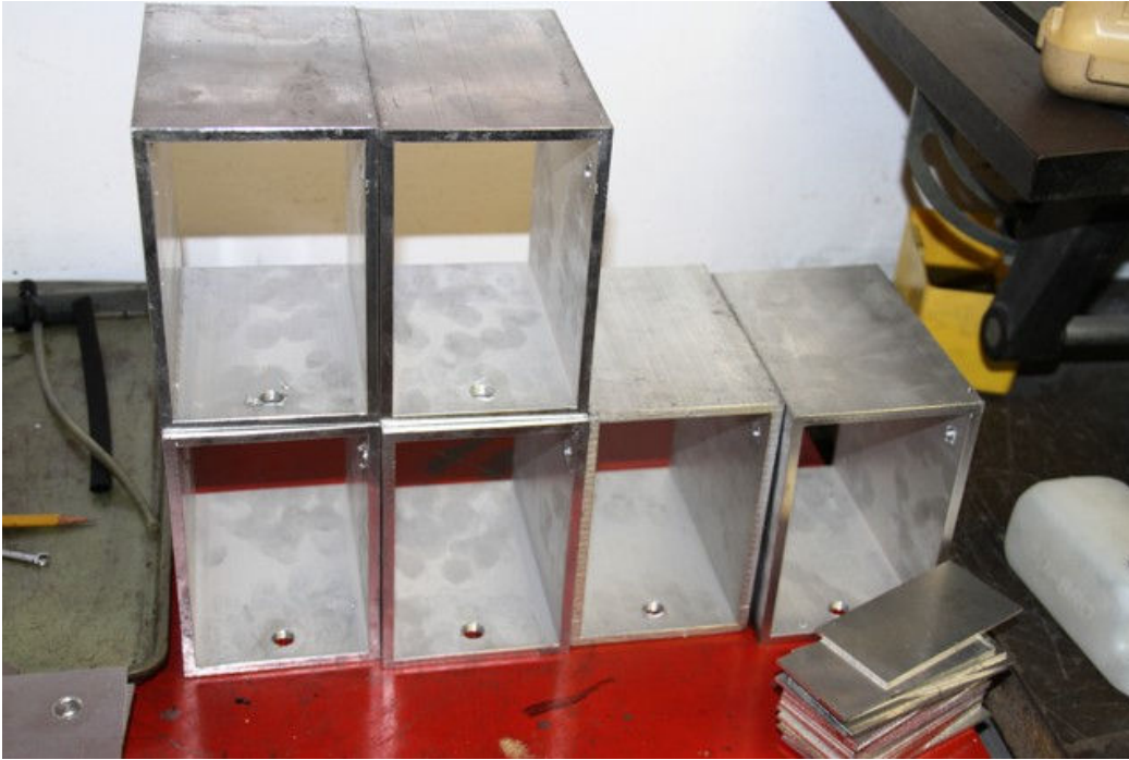
Pic #4 (Water tanks after welding)
