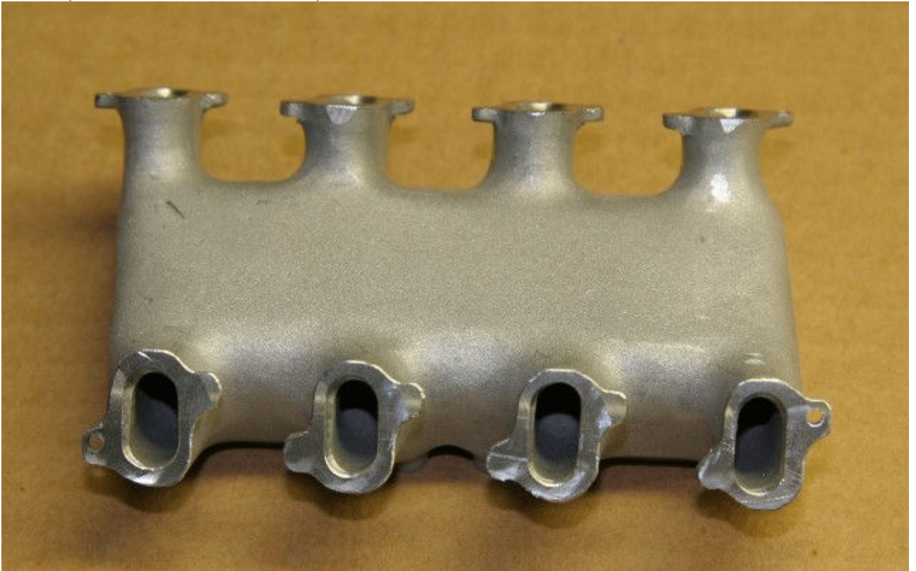
Pic #3 (Bottom on intake manifold)
