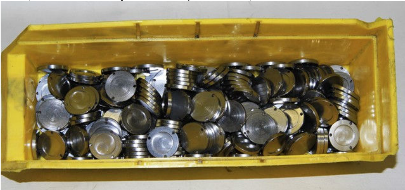
Pic #3 (Rear camshaft covers – polished and ready for installation)
