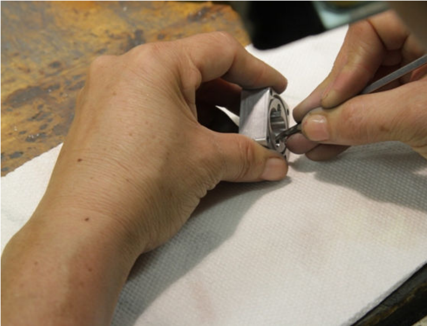
Pic #8 (De-burring oil pump housing)
