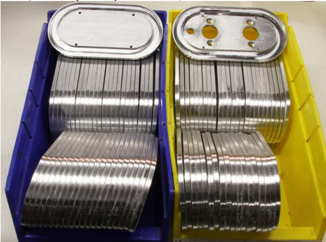
Pic #2 (Air cleaner parts ready for media blast)
