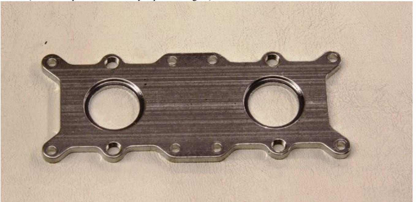
Pic #8 (New base plate for normally aspirated engine)
